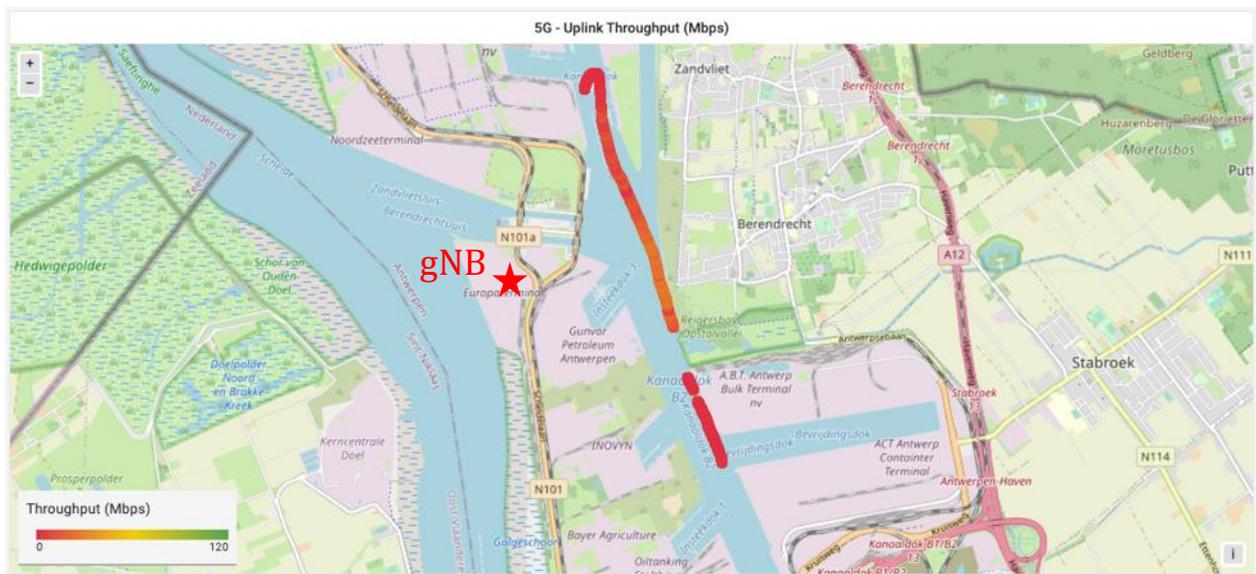
Figure 65: 5G SA TCP uplink rate on map at PoA right bank side
