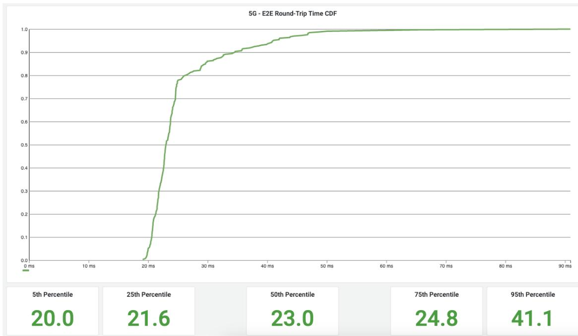
Figure 176: 5G NSA RTT - CDF graph and percentiles at Kloosterboer Terminal 1
