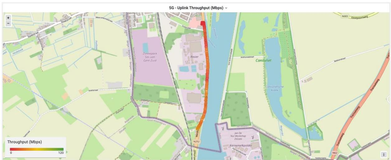
Figure 35: 5G SA TCP uplink rate heatmap during an indicative test at the cross-border site
