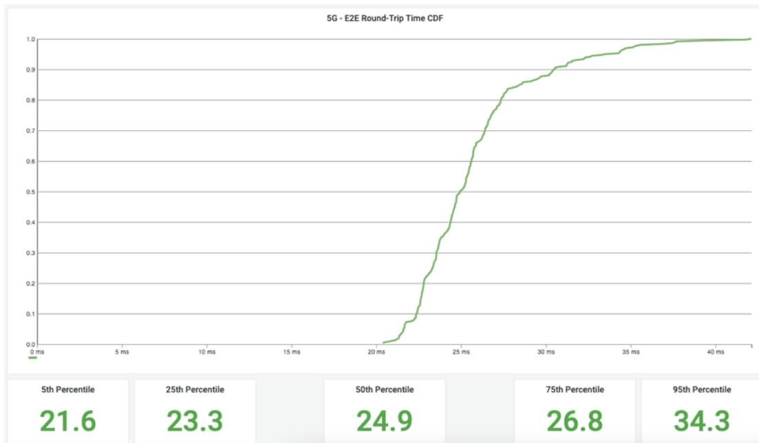
Figure 203: 5G NSA RTT - CDF graph and percentiles at the milk run between the central gate and the Verbrugge Terminals
