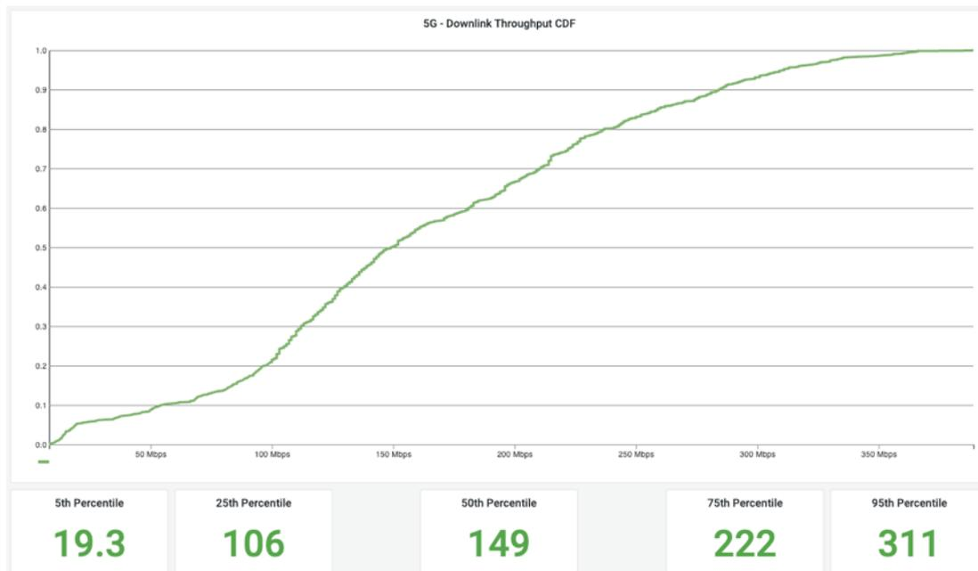
Figure 195: 5G NSA TCP downlink rate - CDF graph and percentiles at the milk run between the central gate and the Verbrugge Terminals
