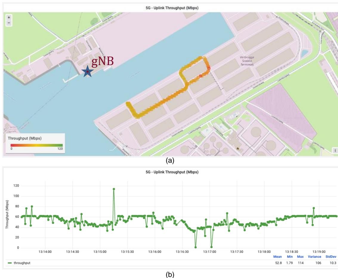
Figure 148: 5G SA TCP uplink rate (a) heatmap, (b) graph throughput vs time – DUT on the eMBB slice without background traffic at Verbrugge Terminals
