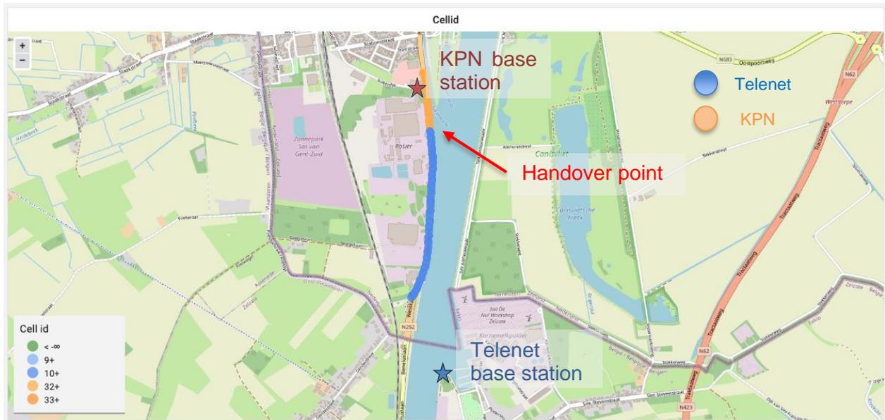
Figure 29: 5G SA attached cell ids during an indicative test at the cross-border site (North to South)
