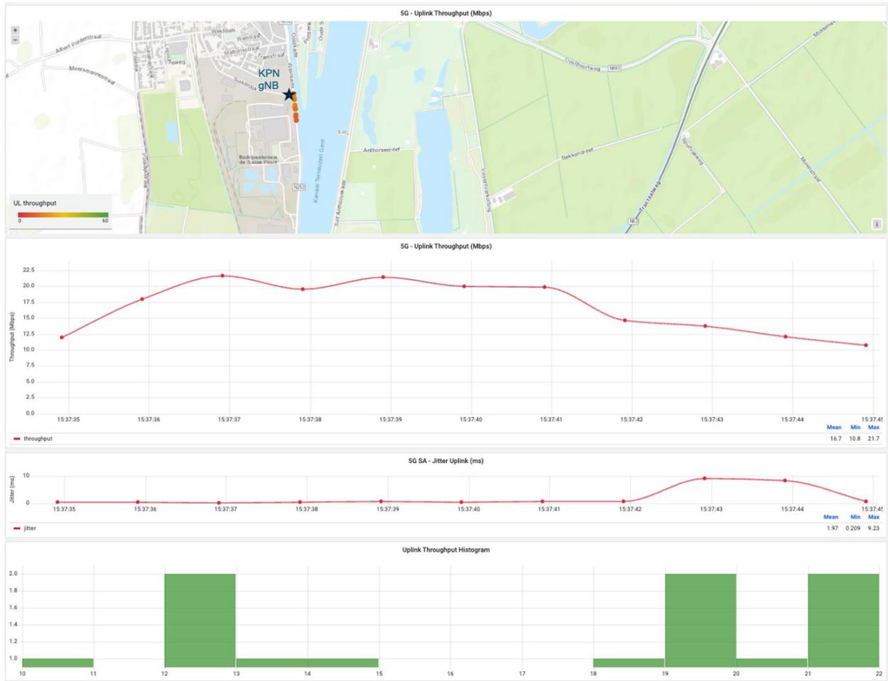
Figure 24: KPN uplink UDP throughput near the gNB on 19/07/23
