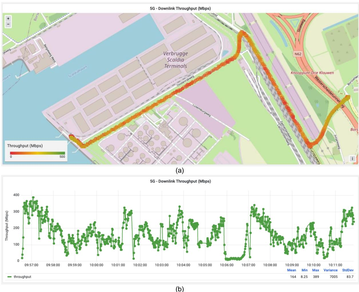
Figure 194: 5G NSA TCP downlink rate (a) on map, (b) graph throughput vs time at the milk run between the central gate and the Verbrugge Terminals
