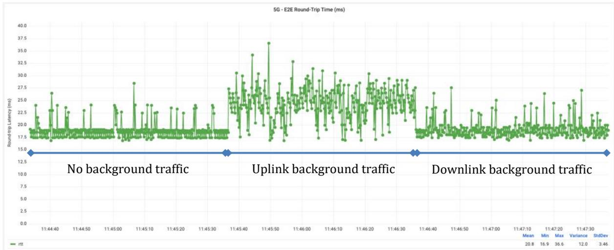
Figure 112: 5G SA RTT – DUT on the URLLC slice and background traffic on the eMBB slice at PoA – on the road
