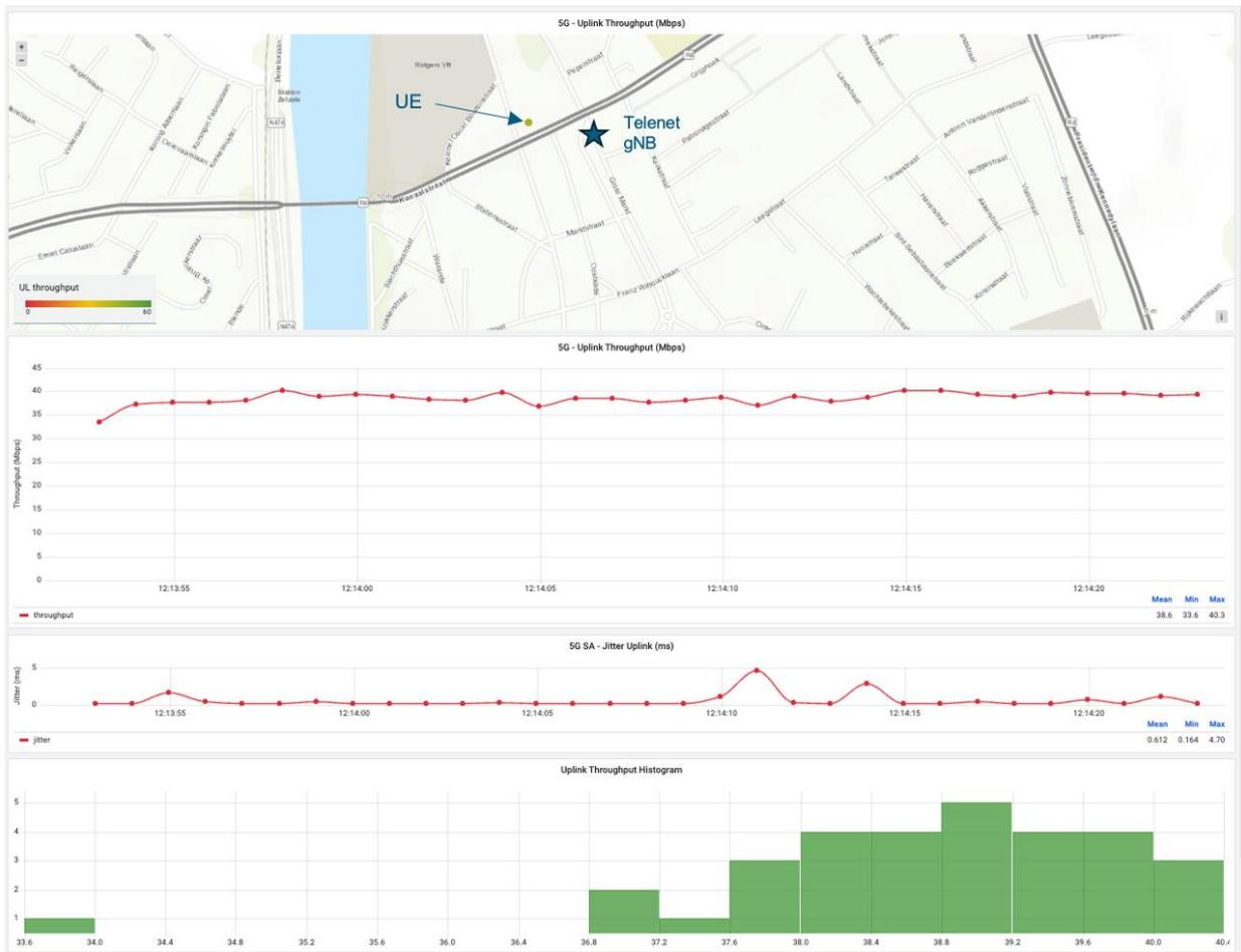
Figure 21: Telenet uplink UDP throughput at Zelzate parking on 19/07/23
