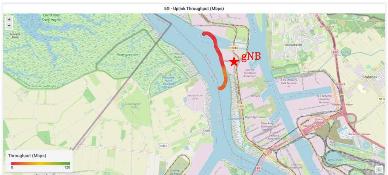
Figure 91: 5G SA - UDP uplink rate on map at PoA Schelde river side
