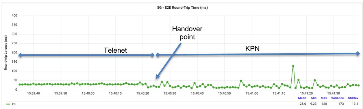
Figure 45: 5G SA RTT graph during an indicative test at the cross-border site
