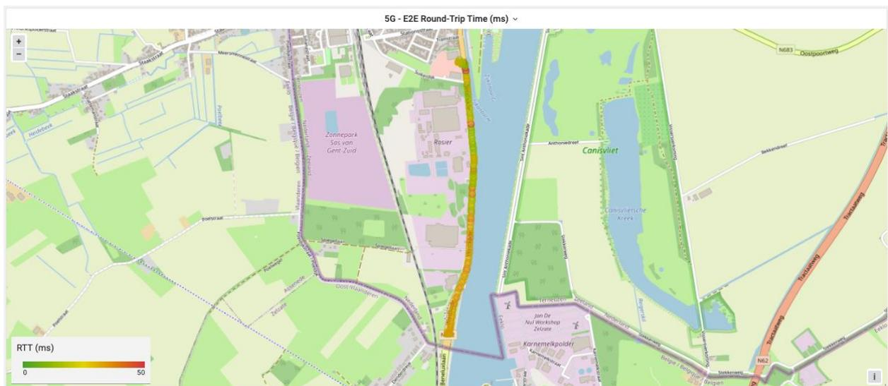
Figure 44: 5G SA RTT heatmap during an indicative test at the cross-border site
