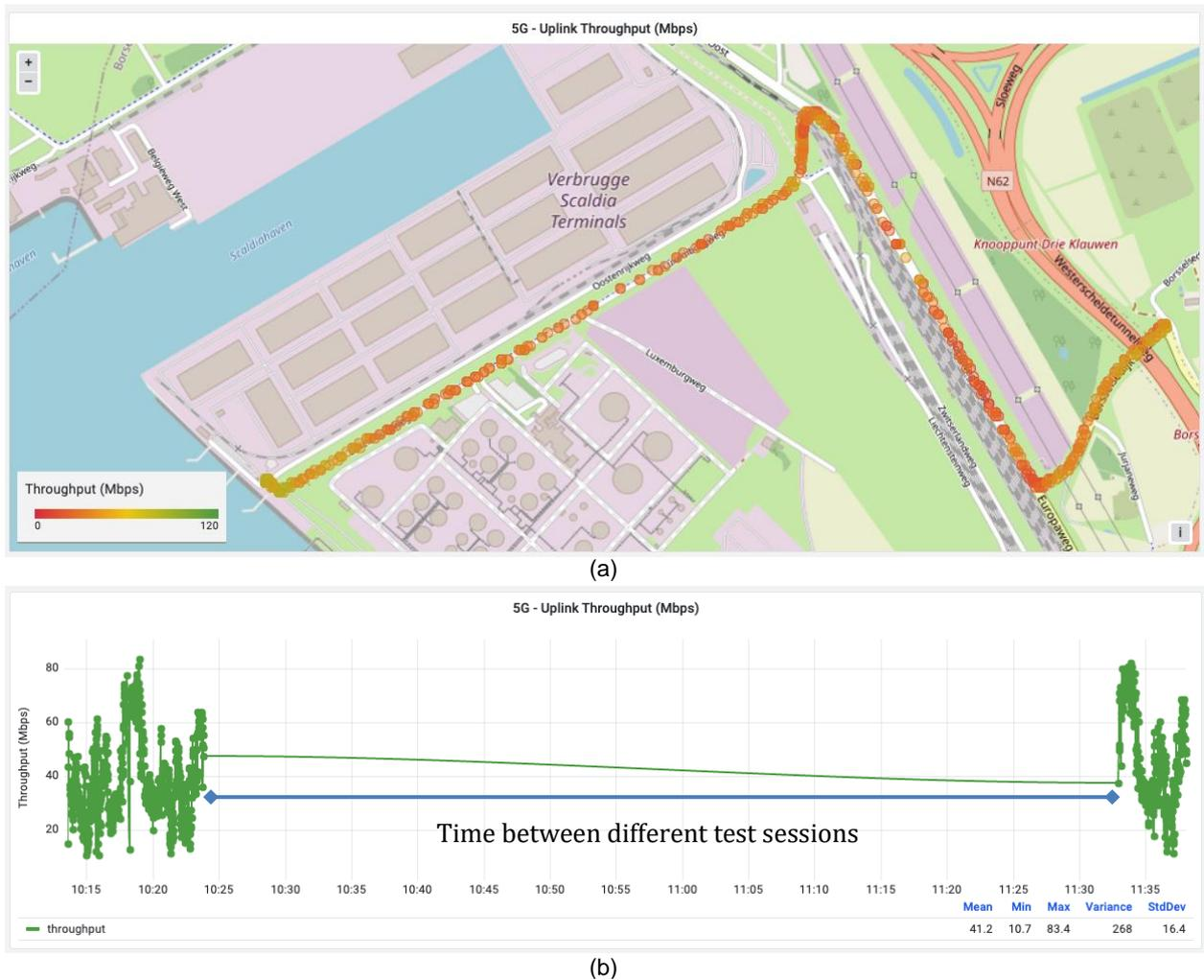
Figure 196: 5G NSA TCP uplink rate (a) on map, (b) graph throughput vs time at the milk run between the central gate and the Verbrugge Terminals
