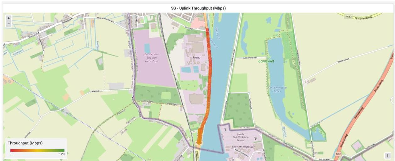
Figure 41: 5G SA UDP uplink rate heatmap during an indicative test at the cross-border site
