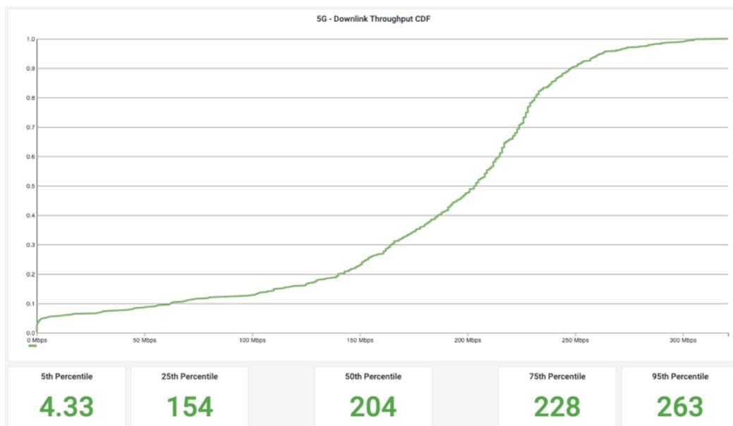
Figure 70: 5G SA UDP downlink rate - CDF graph and percentiles at PoA right bank side
