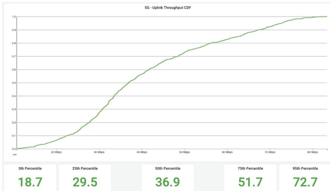
Figure 197: 5G NSA TCP uplink rate - CDF graph and percentiles at the milk run between the central gate and the Verbrugge Terminals
