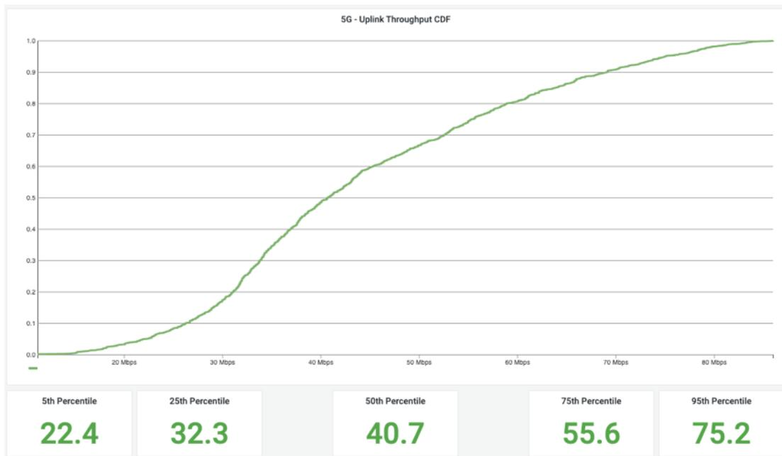
Figure 201: 5G NSA UDP uplink rate - CDF graph and percentiles at the milk run between the central gate and the Verbrugge Terminals
