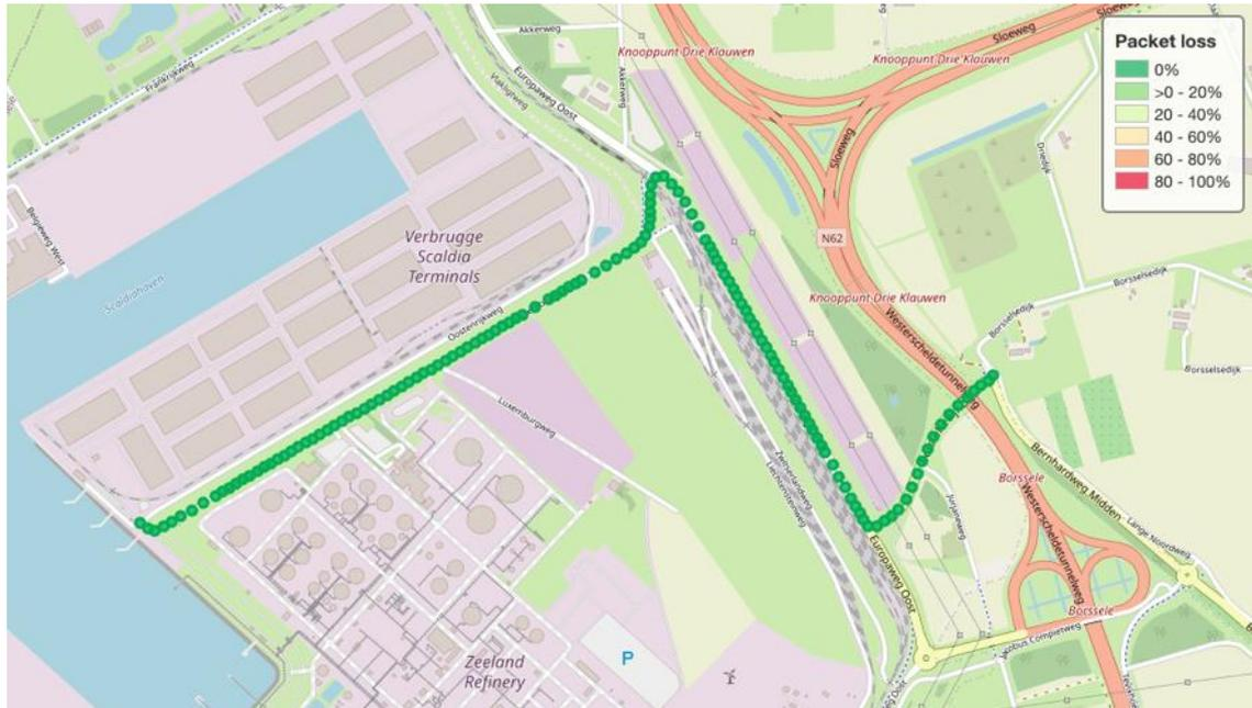
Figure 205: 5G NSA packet loss at the milk run between the Central Gate and the Verbrugge terminal
