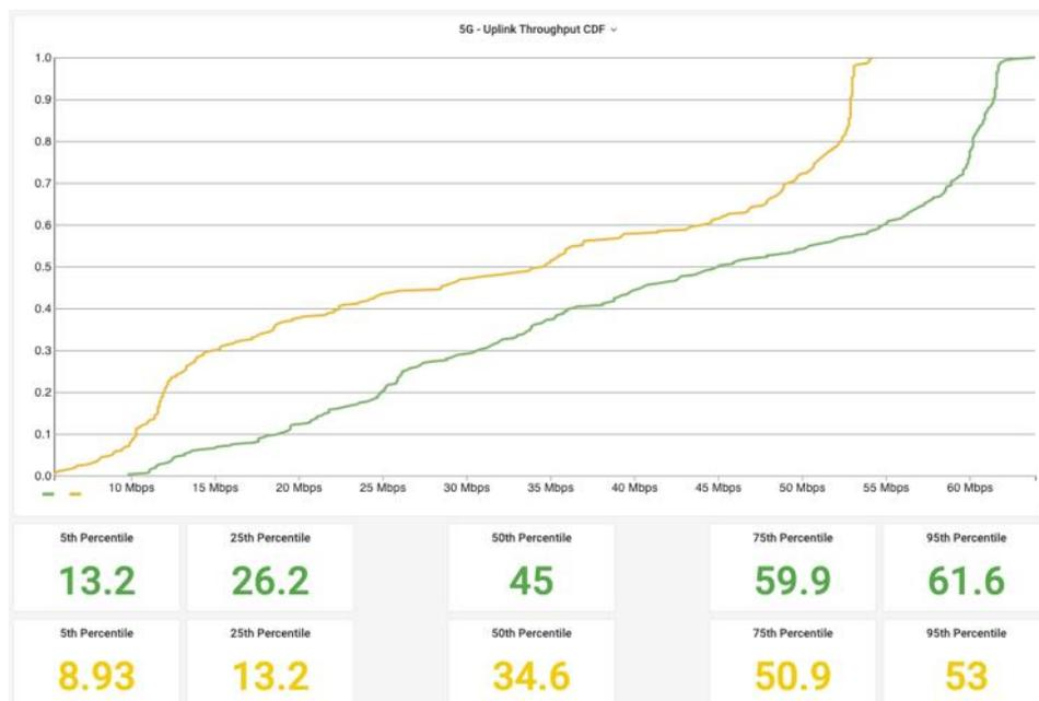
Figure 159: 5G SA UDP uplink rate – DUT on the URLLC slice, without background traffic (green color), with background traffic on the eMBB slice (orange color)
