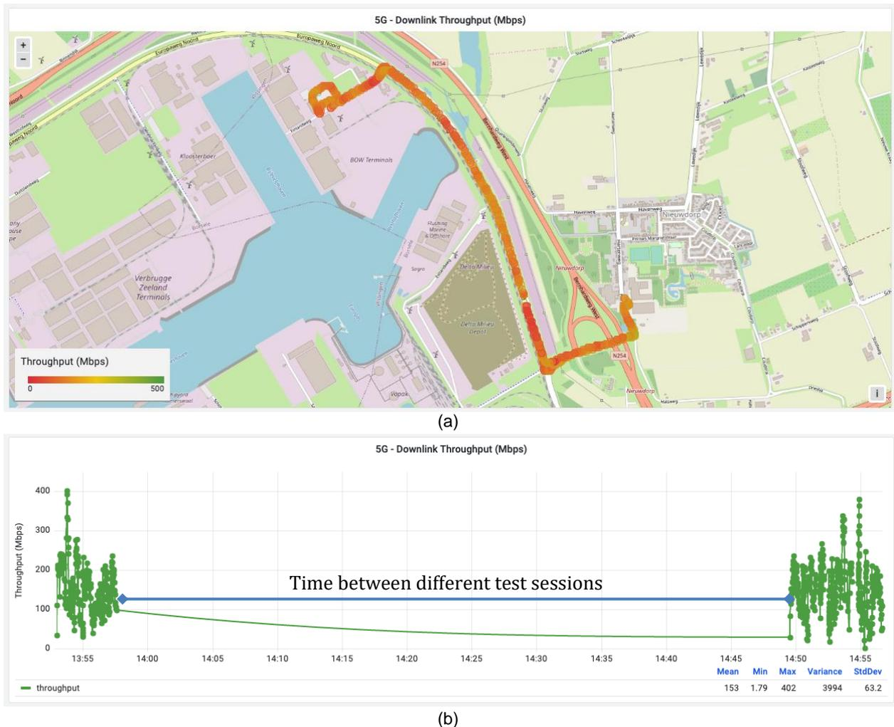
Figure 207: 5G NSA TCP downlink rate (a) on map, (b) graph throughput vs time at the milk run between the Kloosterboer Terminals and MSP Onions
