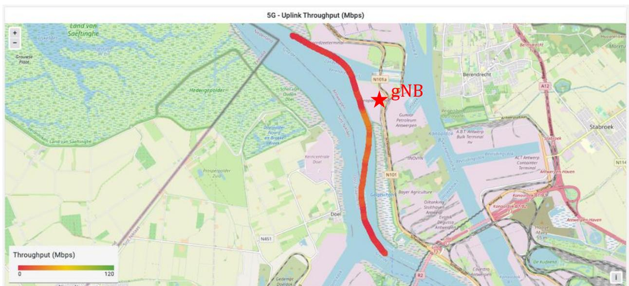
Figure 85: 5G SA - TCP uplink rate on map at PoA Schelde river side
