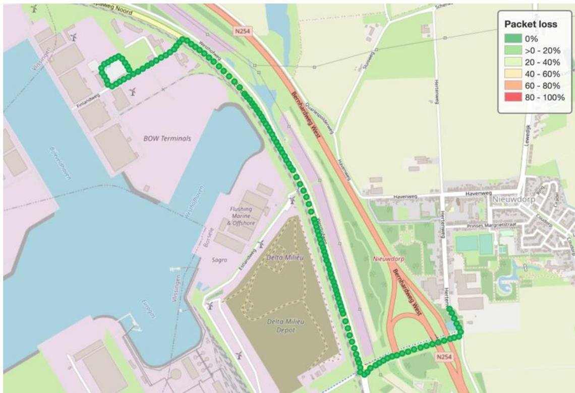
Figure 218: 5G NSA packet loss at the milk run between the Kloosterboer Terminals and MSP Onions
