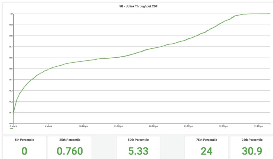
Figure 126: 5G SA UDP uplink rate - CDF graph and percentiles at the Roossens Transport Site
