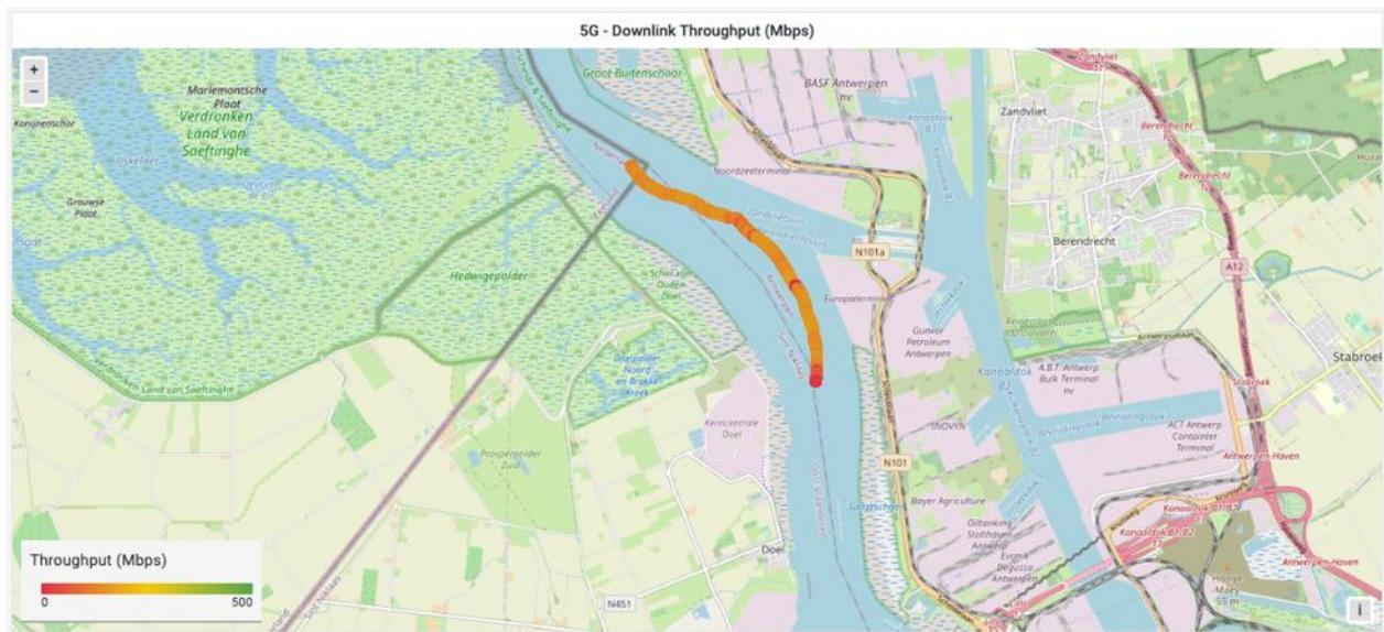
Figure 88: 5G SA - UDP downlink rate on map at PoA Schelde river side
