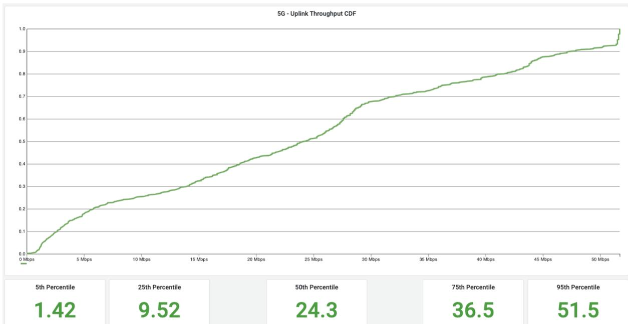
Figure 37: 5G SA TCP uplink rate CDF and percentiles for all the respective tests at the cross-border site
