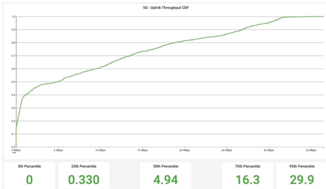
Figure 67: 5G SA TCP uplink rate - CDF graph and percentiles at PoA right bank side
