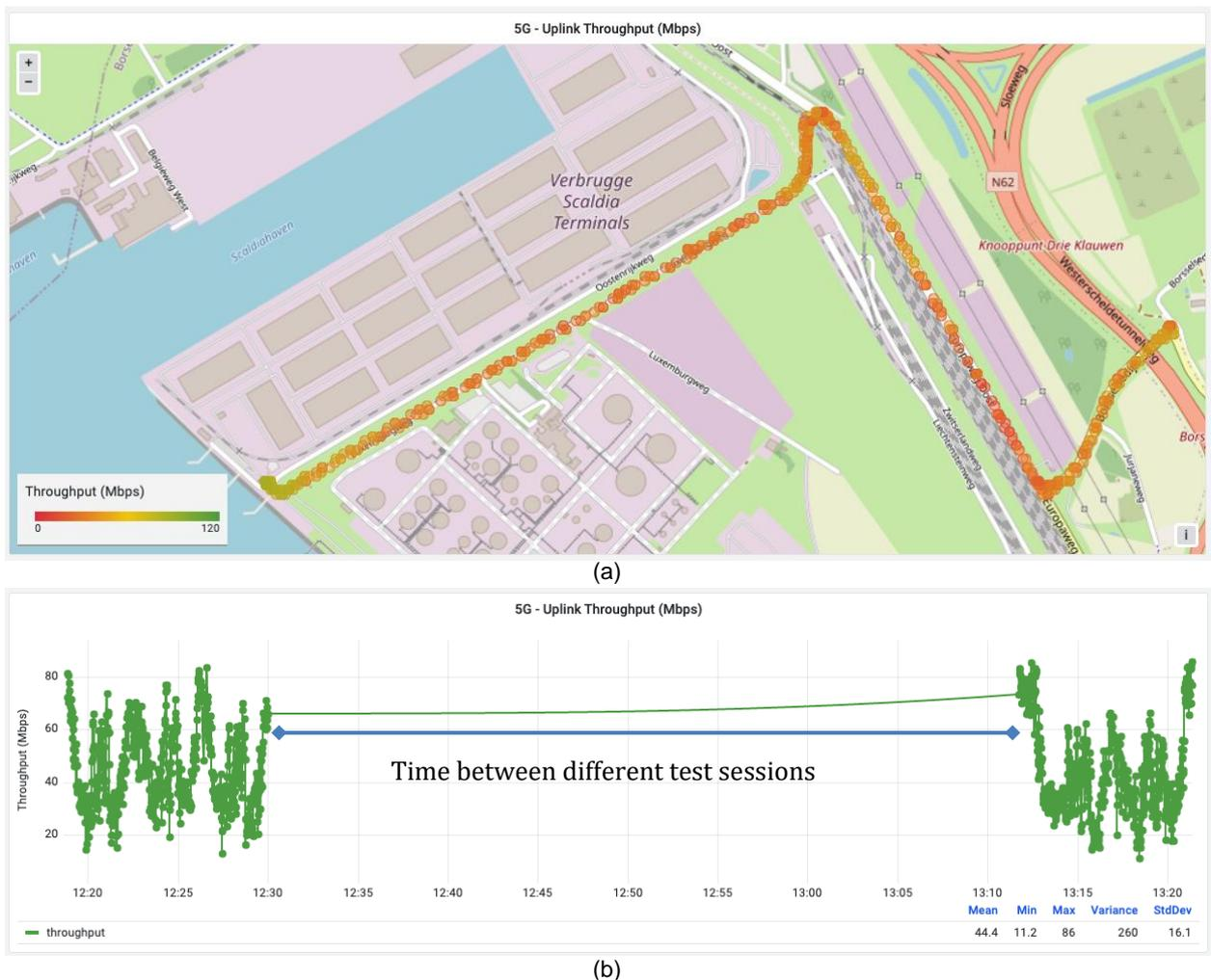
Figure 200: 5G NSA UDP uplink rate (a) on map, (b) graph throughput vs time at the milk run between the central gate and the Verbrugge Terminals
