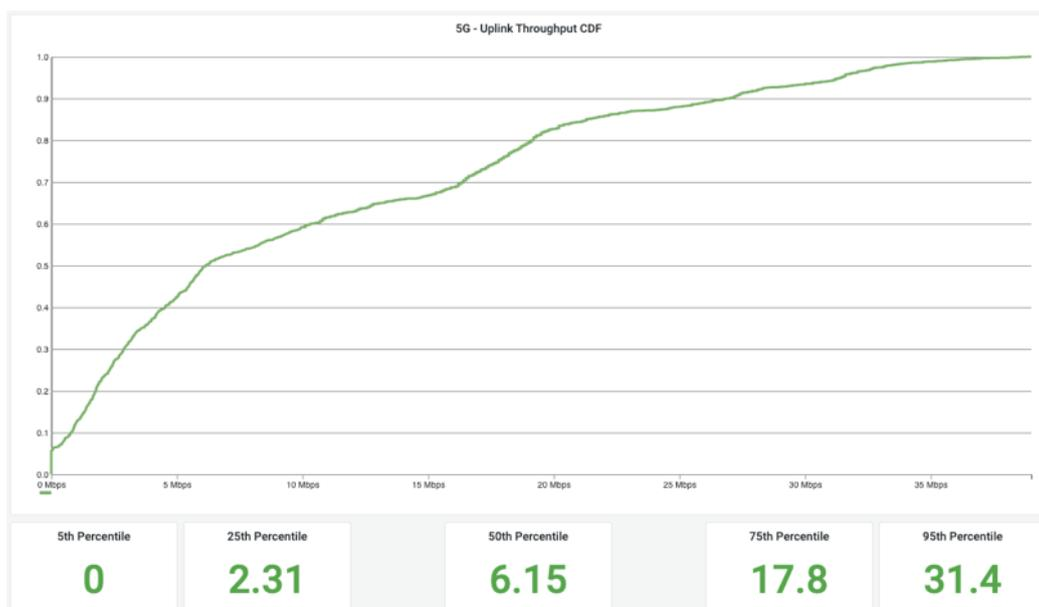
Figure 87: 5G SA TCP uplink rate - CDF graph and percentiles at PoA Schelde river side
