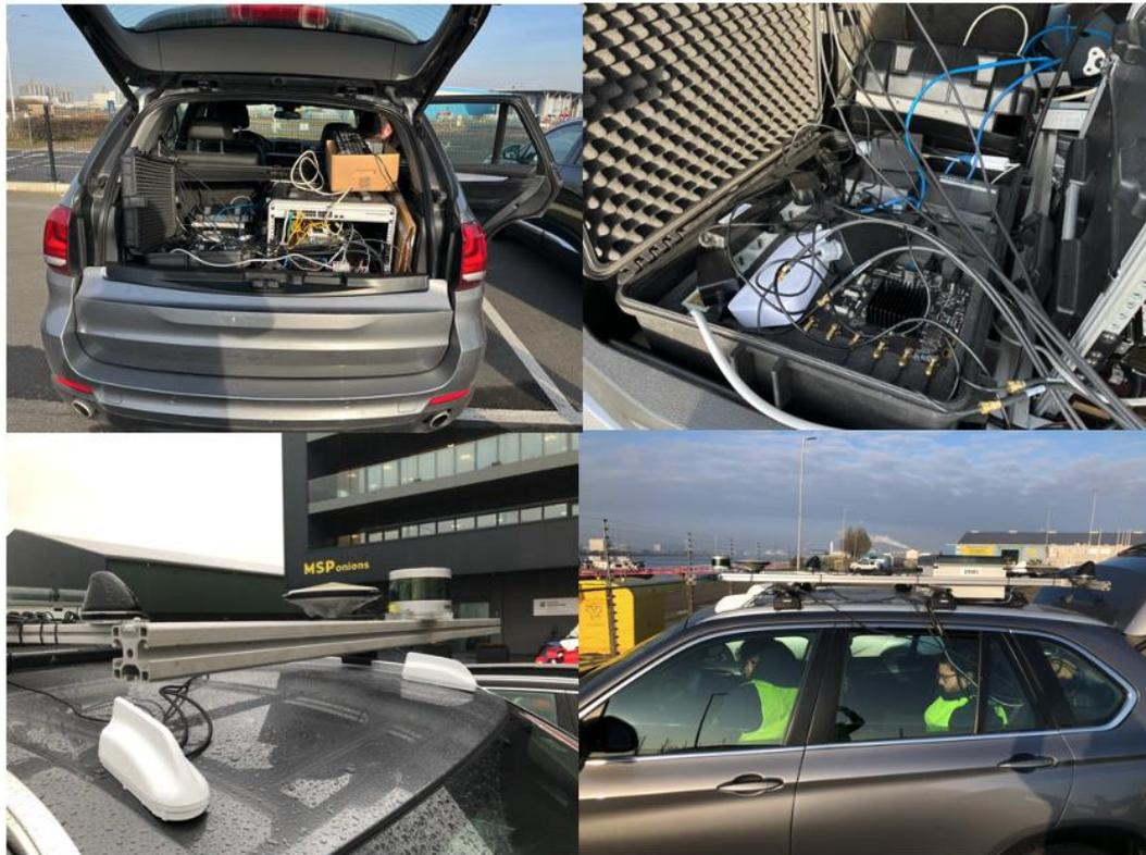
Figure 3: IMEC BMW test car with measuring equipment
