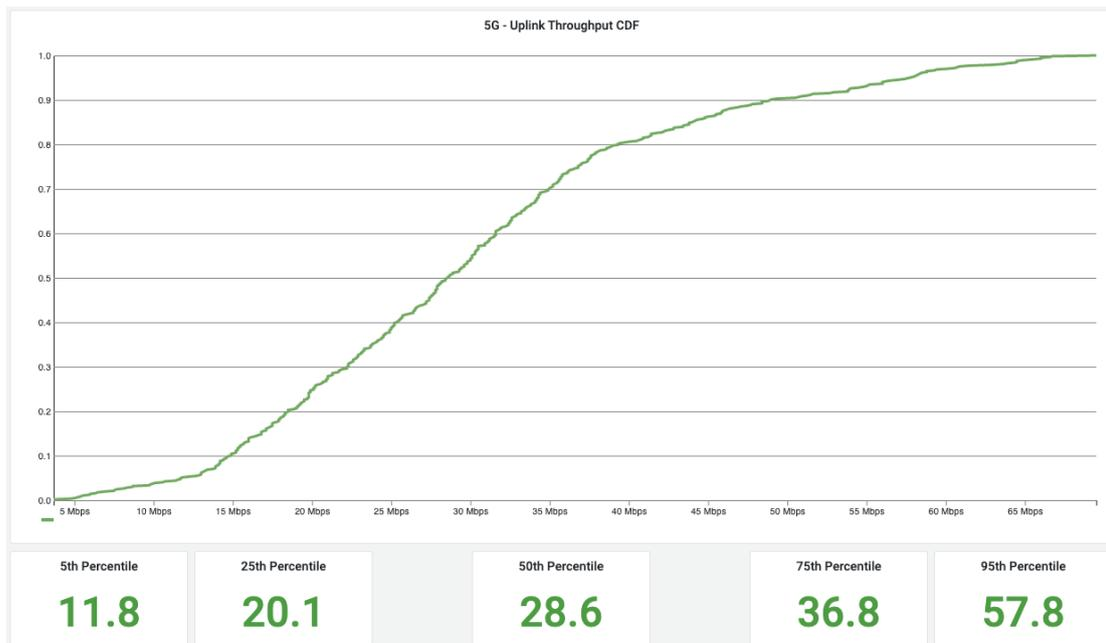
Figure 210: 5G NSA TCP uplink rate - CDF graph and percentiles at the milk run between the Kloosterboer Terminals and MSP Onions
